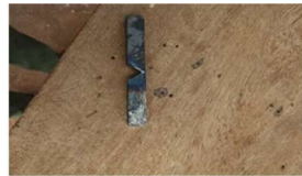
(b) Cut V-butt joint
