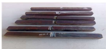
Figure 5: Impact strength test specimens
