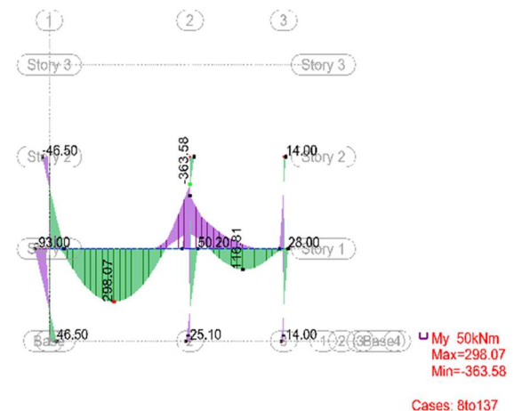
Figure 7: Subframe Bending Moment Envelope for Model S at 0.25 m mesh size
