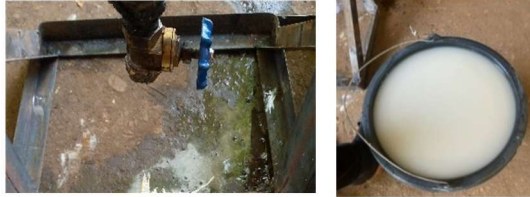
Plate 6. Discharge Chute for cassava slurry collection
