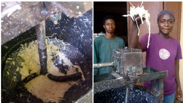
Plate 9. Stirrer arms inside the separating drum
