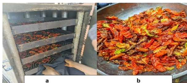
Figure 4: The drying process of pepper (a) is the pepper inside the dryer (b) is the dried pepper.
