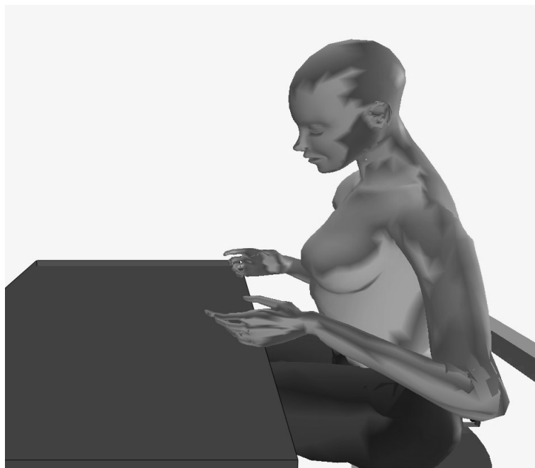
Figure 2: Incorrect, Too High Position of the Table Top Surface (Source: Źabińska et al., 2018).
