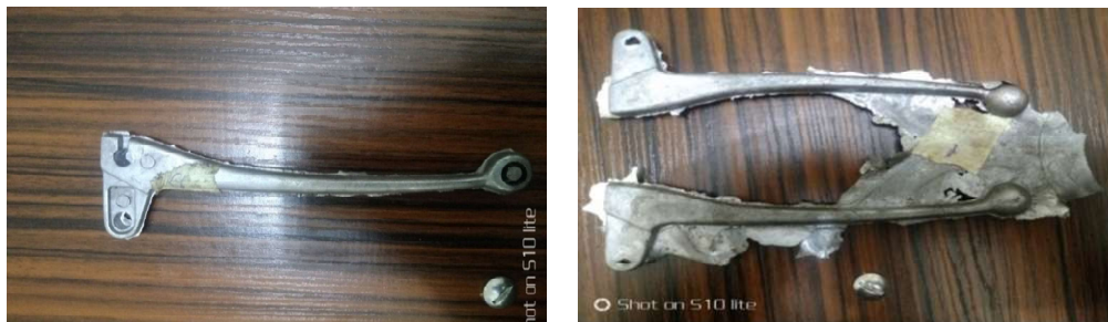
Plate 3: Cast component of motorcycle brake handle
