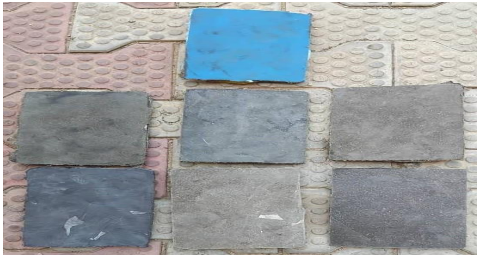
Figure 4: Visual representation of the composite sample formed through the combination of rLDPE, sawdust, natural rubber and other additives.
