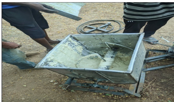
Plate 2. Dough mixing using the fabricated machine.
