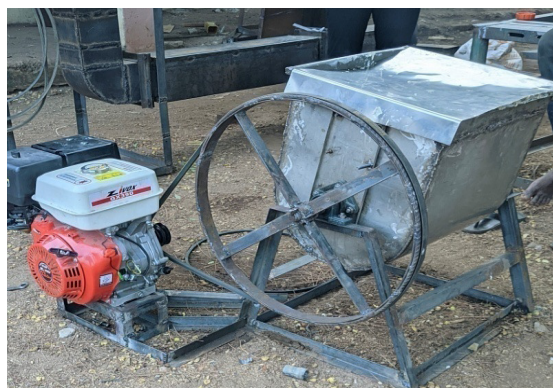
Plate 1: The developed engine powered horizontal mixing machine.
